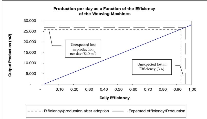
**Figure 4** – The Impact of an “Unexpected” Loss in the Efficiency of the New Weaving Machines on the Daily Production of the Weaving Mill.
