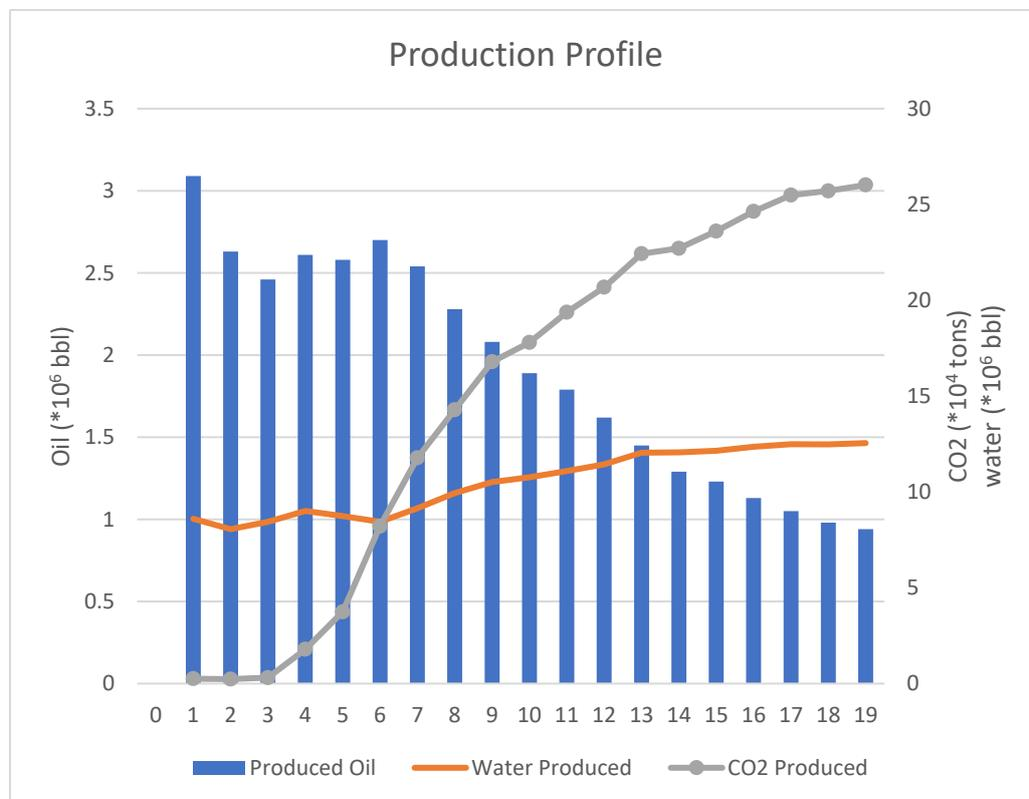
Figure 7: Reservoir Simulation Showing Oil, Water and CO<sub>2</sub> production data
